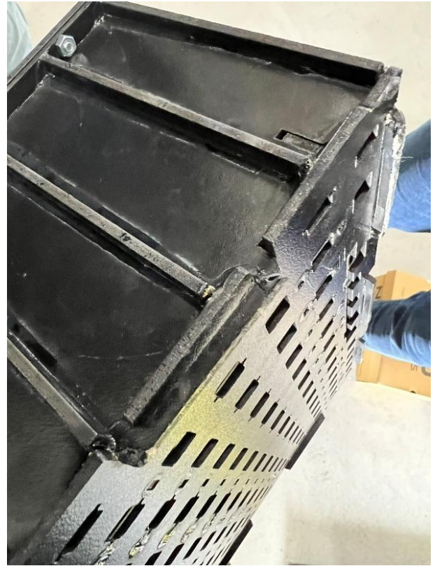
b) Damage after LC2
