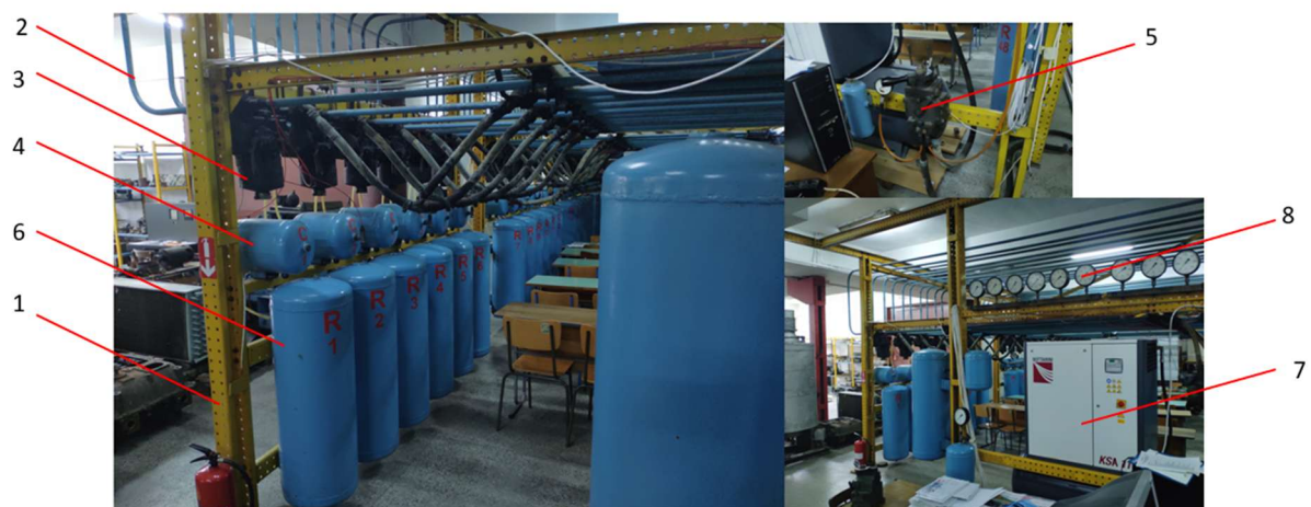
Fig. 2.1 General view of the gas-dynamic test rig for braking systems: 1 – supporting structure; 2 – air pipes (brake pipe); 3 – distributor valve type KE1; 4 – brake cylinder; 5 – driver's brake valve Knorr D2; 6 – auxiliary reservoir; 7 – compressor; 8 – pressure gauges.
