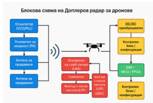
Fig. 3.1. Sample block diagram of a 24 GHz radar, suitable for Doppler or FMCW (Frequency-Modulated Continuous Wave) radar (diag. – AI)
