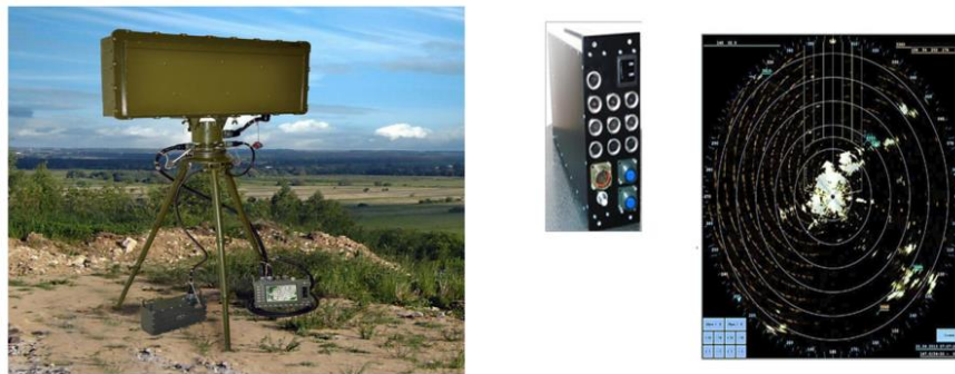
Fig. 3.31. 3D radar with a phased antenna array, plot extractor, and plan position indicator (PPI).
