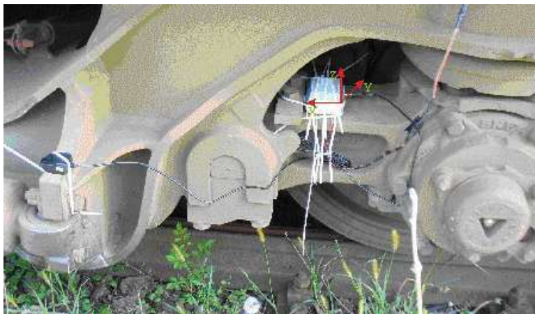
Fig. 5.12. Measuring device mounted on a axle box
